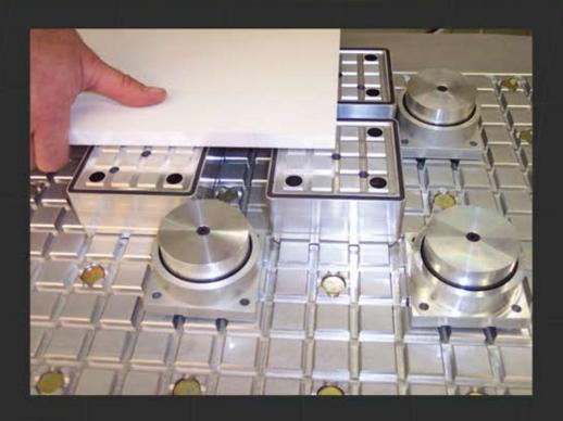
THE NEMI GRID TABLE VACUUM FIXTURING SYSTEM IS DESIGNED TO HOLD YOUR PARTS SECURE USING VACUUM. THE SYSTEM CONSISTS OF A VACUUM GRID TABLE, VACUUM PODS, AND LOCATOR PINS. SIMPLY REMOVE THE WASHERS FROM THE GRID TABLE WHERE YOUR PODS AND LOCATORS PINS WILL BE POSITIONED, PLACE YOUR PODS AND LOCATOR PINS ON THE GRID TABLE, LOCATE YOUR MATERIAL ON THE PODS AGAINST THE PINS, TURN ON YOUR VACUUM AND YOU ARE READY TO GO. THE LOCATOR PINS DROP DOWN AND THE VACUUM PODS HOLD YOUR PARTS SECURE.
