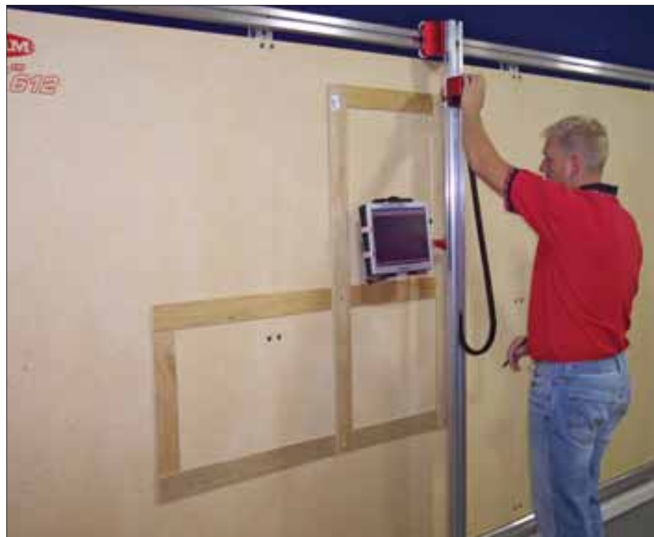
Jason Akre demonstrates how easy and efficient the NEMI DigiCoder™ is to use. The NEMI DigiCoder™ is currently the only digitizer on the market with a trace function. Templates and parts that used to take two weeks to calculate geometrically may now be produced in as an hour to produce a .DXF file.
